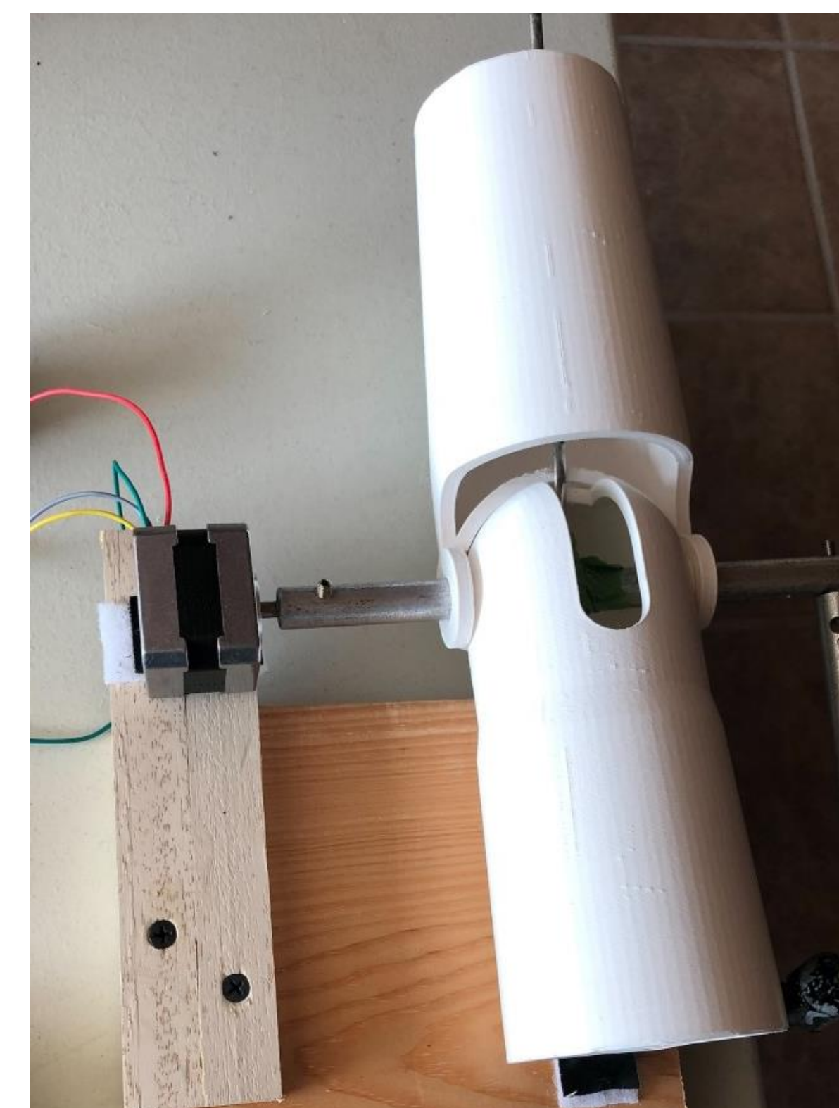
Figure 1. Setup of elbow joint with the stepper motor attaching the upper arm and lower part of the arm together.
