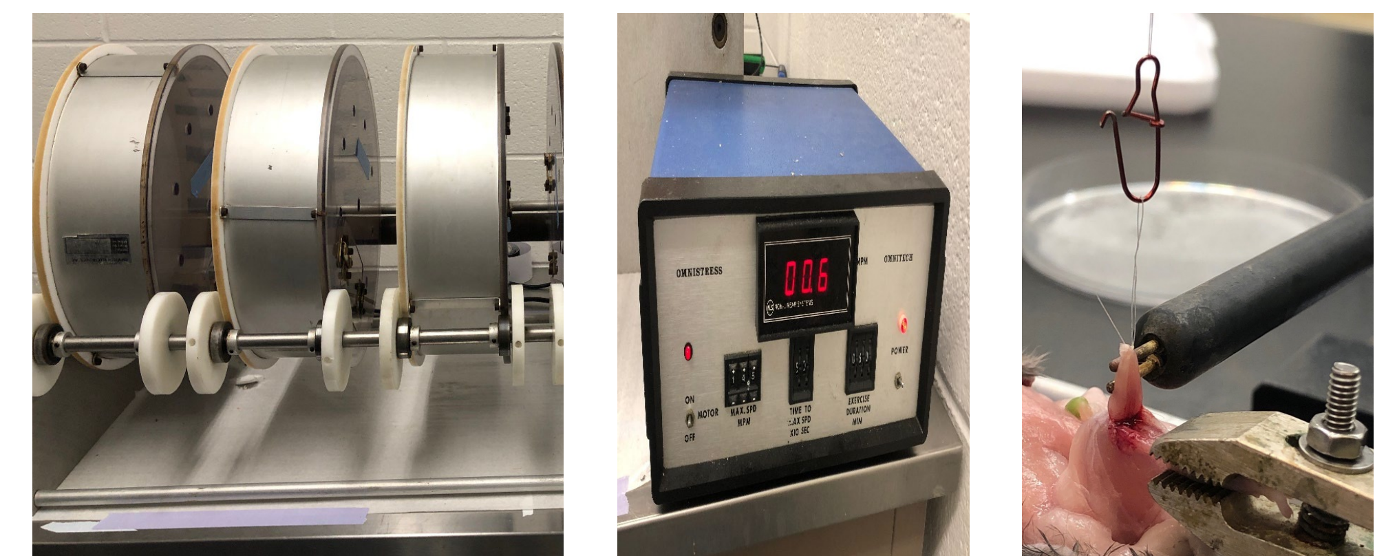
Figure 1. The mouse treadmill apparatus had 5 wheels driven by an electric motor. We were able to control: max speed in meters per minute (mpm), time to max speed X10 seconds, and exercise duration in minutes. We gradually increased max speed and exercise duration over the course of 4 weeks for the exercise group as indicated in Table 1. Control and High Fat groups did not run on the treadmill. All animals received ad libitum water and food for the duration of the experiments.
