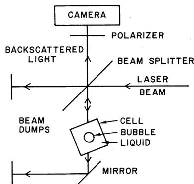
FIG. 2. Apparatus for observing backscattering from bubbles.
