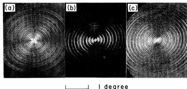
FIG. 3. Photographs for (a) crossed polarizer ( $l=2$  scattering); (b) uncrossed polarizer ( $l=1$ ); and (c) no polarizer. The incident polarization was vertical.  $a = 0.49$  mm and  $x = 6830$ .
