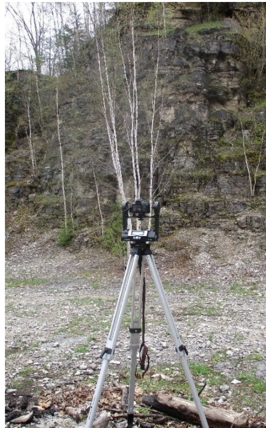
Figure 1. Image of GigaPan® system in use at Scott Quarry. A digital camera is mounted inside the GigaPan® motorized mount, which itself is attached to an aluminum tripod.
