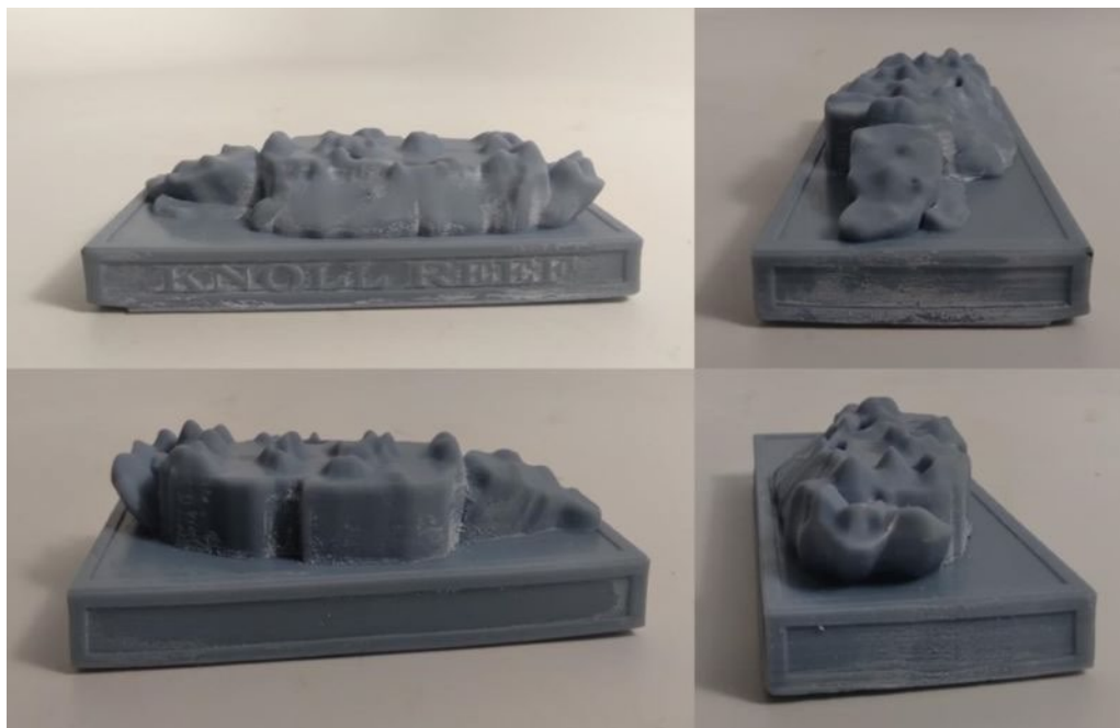
Figure 8. The four sides of the knoll reef 3D print at a scale of 60:1.
