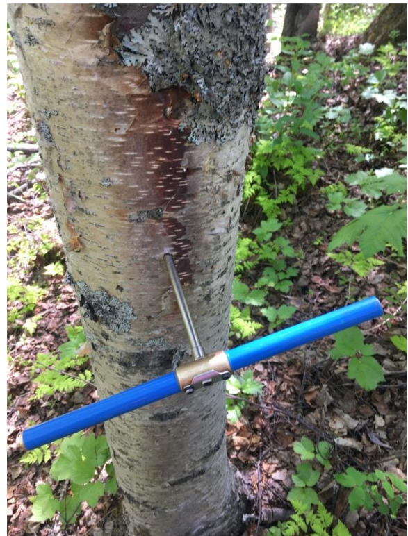
Figure 4. Increment borer in an Alaska paper birch with spoon and sample extracted.
