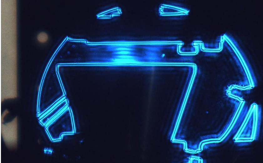
Figure 12: Adjusting the separation distance at 11.77 mm a few millimeters further from the levitator shifts the high-pressure zone to the middle of the levitator.
