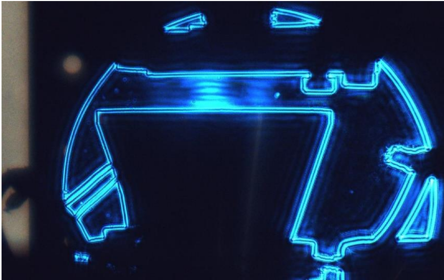
Figure 16: Shifting the standing waves towards the middle of the levitator at 11.77 mm by decreasing the separation distance by fractions of a millimeter. The high-pressure zones are bright blue while the low-pressure zones are dark blue to black.
