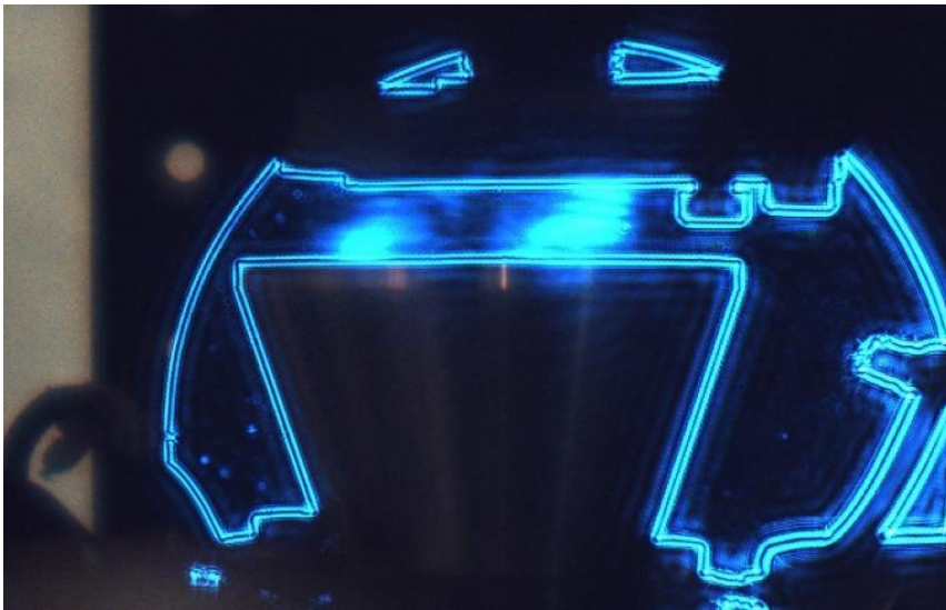
Figure 13: The standing waves created at a separation distance of 11.77 mm. The high-pressure zones are bright blue while the low-pressure zones are dark blue to black.
