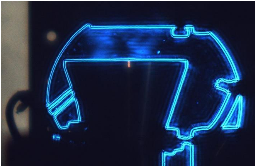
Figure 19: The standing waves created at a separation distance of 19.46 mm. The high-pressure zones are bright blue while the low-pressure zones are dark blue to black.
