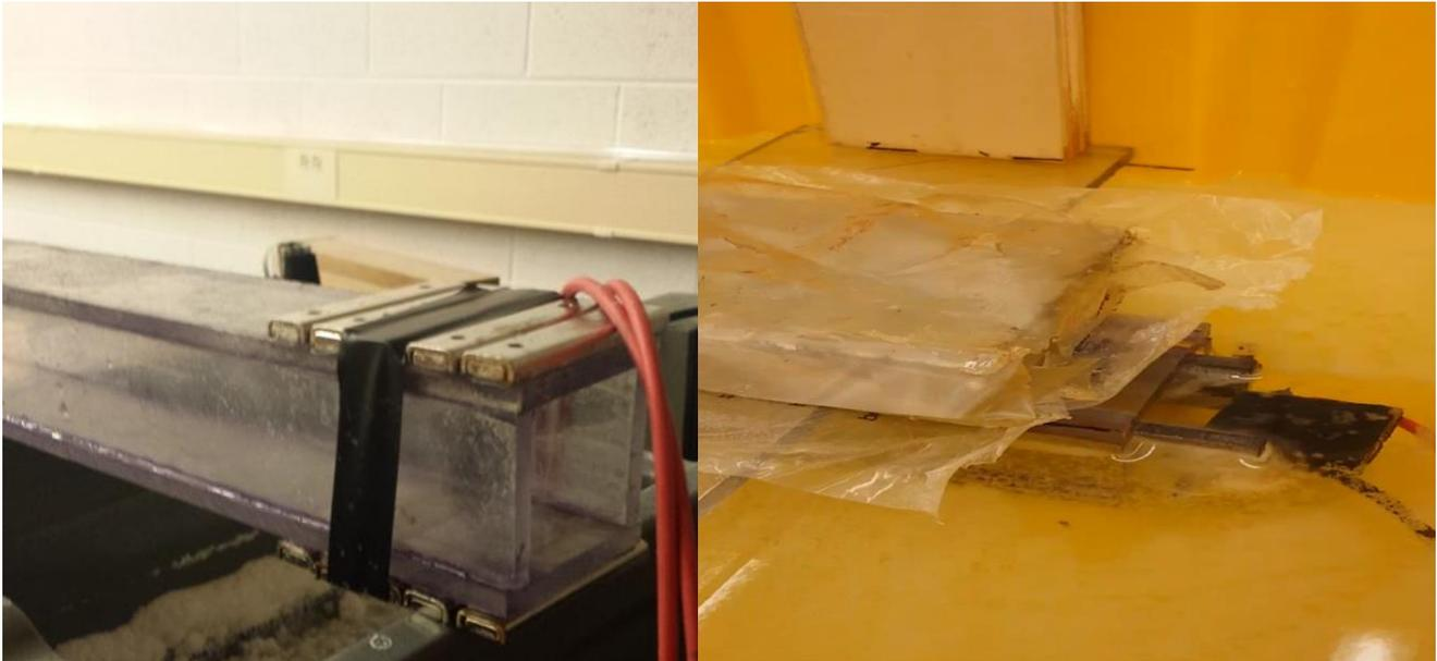
tube made from acrylic (Figure 2). With this setup, I was able to see a weak flow of roughly one centimeter per second. I then moved to scale up the magnetic field and to have a more regulated voltage source. Using the same acrylic tube with new electrodes and stronger magnets, I had my final prototype.
