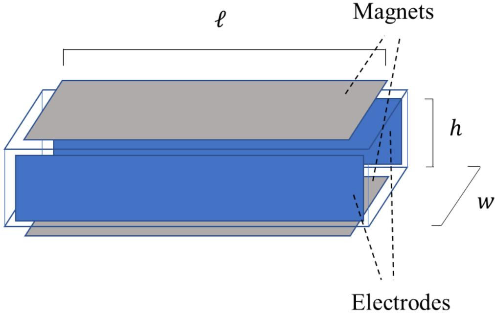
Figure 5: Tube dimensions diagram.
