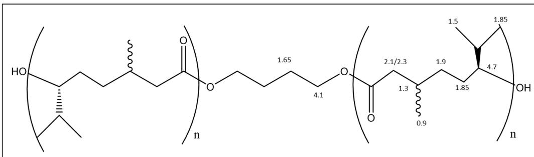
Fig. 2.5.  $^1\text{H}$  NMR assignments for PM.
