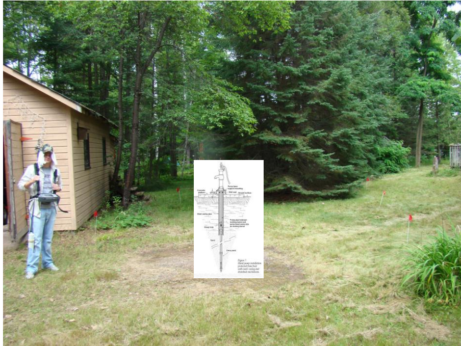
Figure 5. 2010 study site. Co-author Kris Neuhauser ready with G-858 cesium magnetometer unit. Plastic flags at 5-meter grid intervals. Inset diagram of a hand pump system with drill spike (WSH, 2012). Photo by K. J. Neuhauser.
