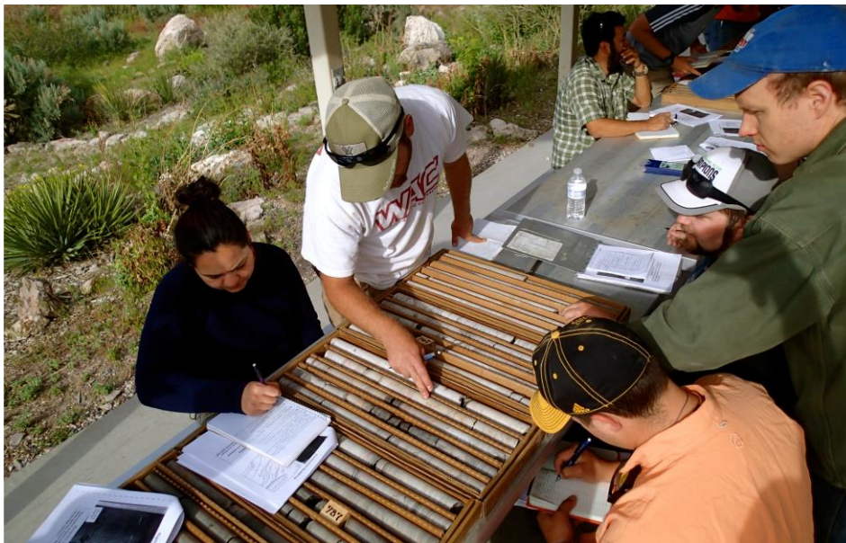
Figure 10. Photo of students evaluating the cores taken from the Books Cliffs area. The cores show the transitions of the layers from the Starpoint Sandstone through to the Castlegate Sandstone. These cores show a changing depositional setting from bay fill, near shore environments to more fluvial
