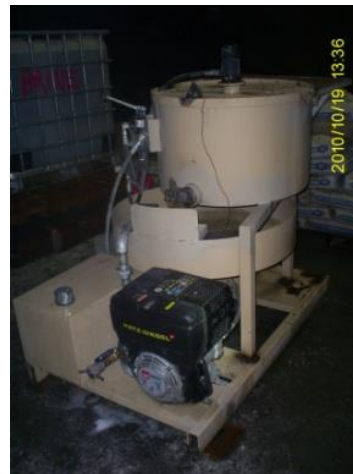
Figure 9. Diesel powered grout pump.
