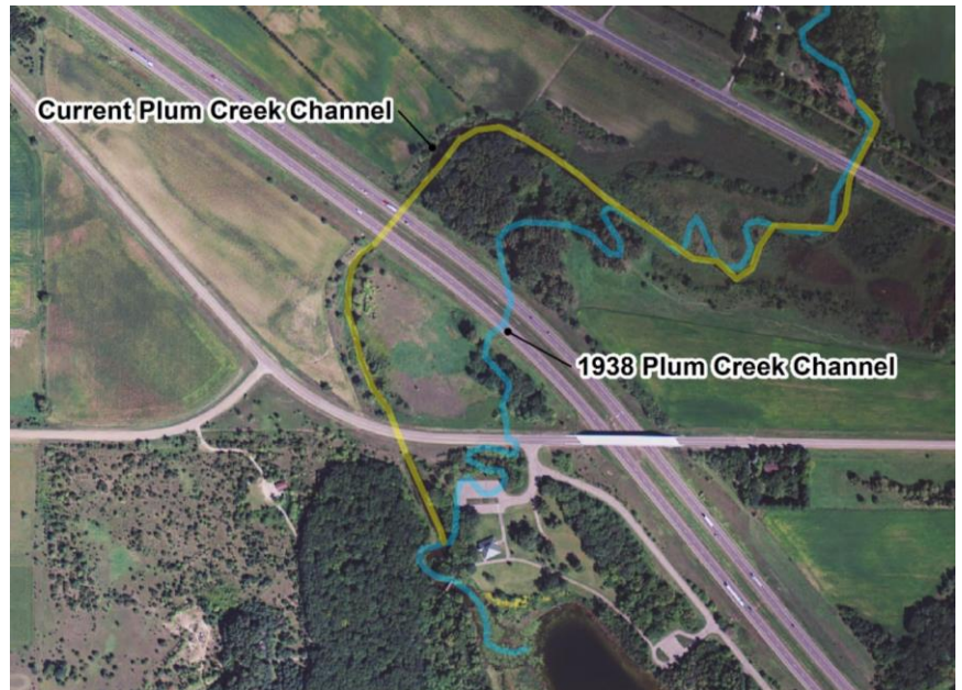
Figure 6. Map of Plum Creek channel construction to accommodate Interstate 94 from Stearns County Soil and Water Conservation District.
