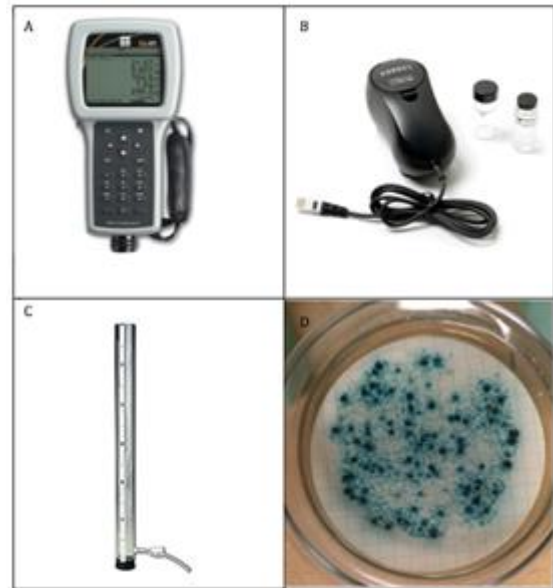
Figure 10. Instrumentation used for this study included (A) Y-Si 556 multi-probe from YSI.com (B) Vernier Turbidity probe from Vernier.com (C) Transparency tube from Grainger.com (D) Incubated membrane filtered sample
