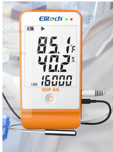
Figure 2: The Elitech GSP-6G data logger with temperature and humidity sensors was used to collect data at the three sites. It was programmed using the software included with purchase that was downloaded from the company website. Using the data loggers required some trial and error to determine an ideal logging interval and the logging could sometimes be interrupted if the sensors got wet or experienced some other interference.
