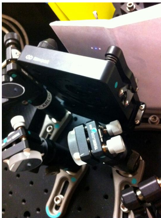
Figure 8. Both of the split 800 nm beams that entered the BBO crystal were overlapped in time and space and can be seen as the two outside red dots on the paper. The 400 nm SHG beam was successfully produced from the overlap and is the middle blue dot.
