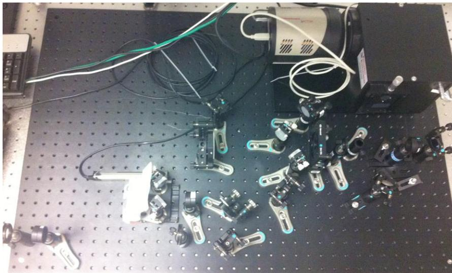
Figure 7. Above is an actual image of the Kansas State University HITS FROG. Fig. 4 is simply a schematic of this setup.
