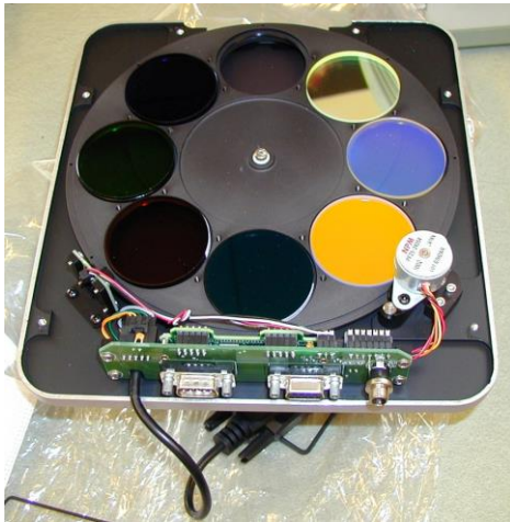
Figure 2: SBIG filter wheel with B, V, I, R, and blank filters; the additional filters (not used) are sloan g' , r' , i' filters.
