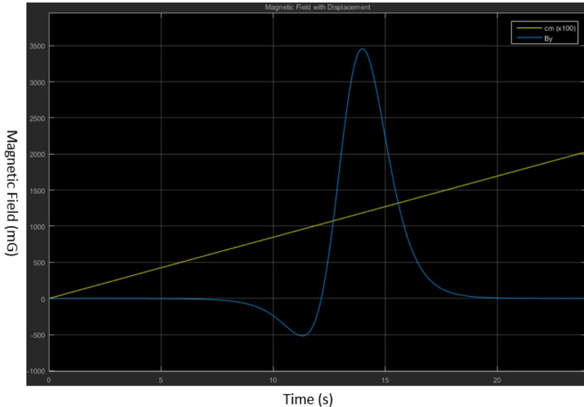
*Figure 6.* Modeled magnetic field data of dipole magnet attached to extending piston of electro-hydraulic actuator compared to the displacement of the piston. This was simulated using Simulink with a simulation run time of 24 seconds as consistent with experimental test times.
