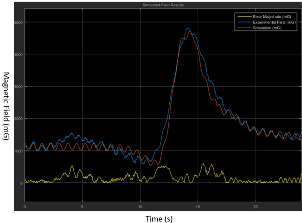
*Figure 7.* Simulated magnetic field compared with experimental data of magnetic field. This 24 second simulation contained modeled disturbances contributed by the DC electric motor superimposed on the baseline dipole magnet field.
