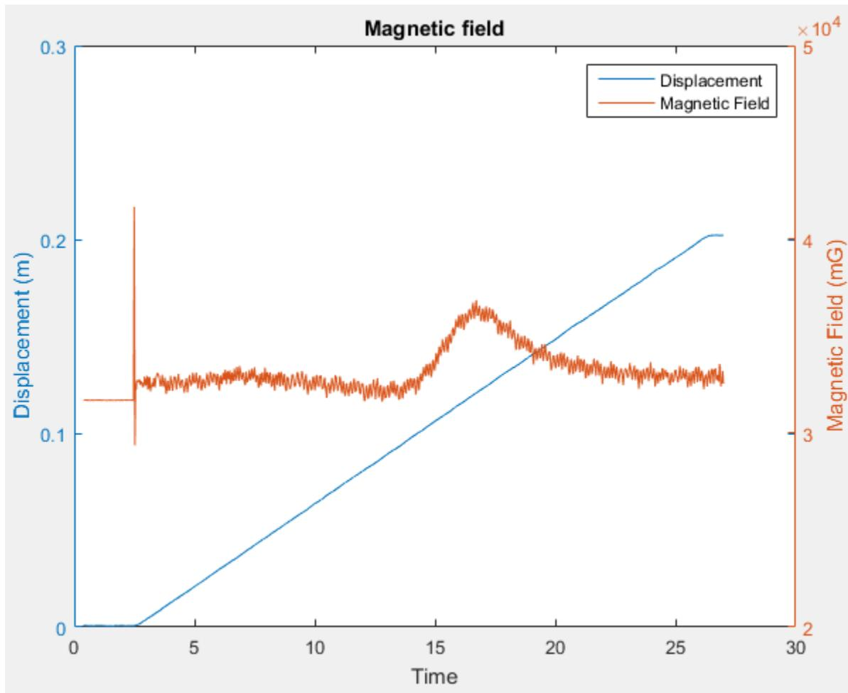
*Figure 4.* Magnetic field data of dipole magnet attached to extending piston of electro-hydraulic actuator compared to the displacement of the piston. The large disturbance at the beginning and end of the 20 second duration test indicates the 12V DC motor initializing/terminating 10A current draw.
