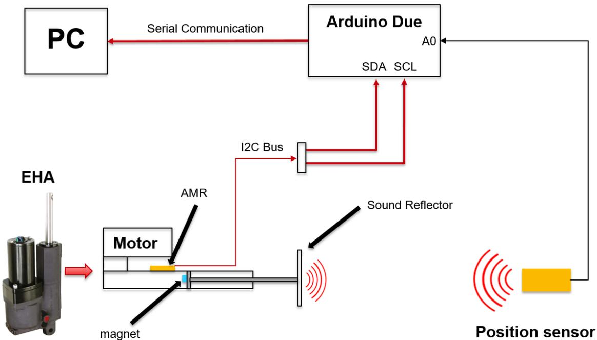
*Figure 1.* Diagram of apparatus used for experimentation. The yellow blocks indicate sensors, the red signal wires indicate serial communication, the black wire indicates an analog signal. Neither of the two power sources driving the EHA or position sensor are shown.
