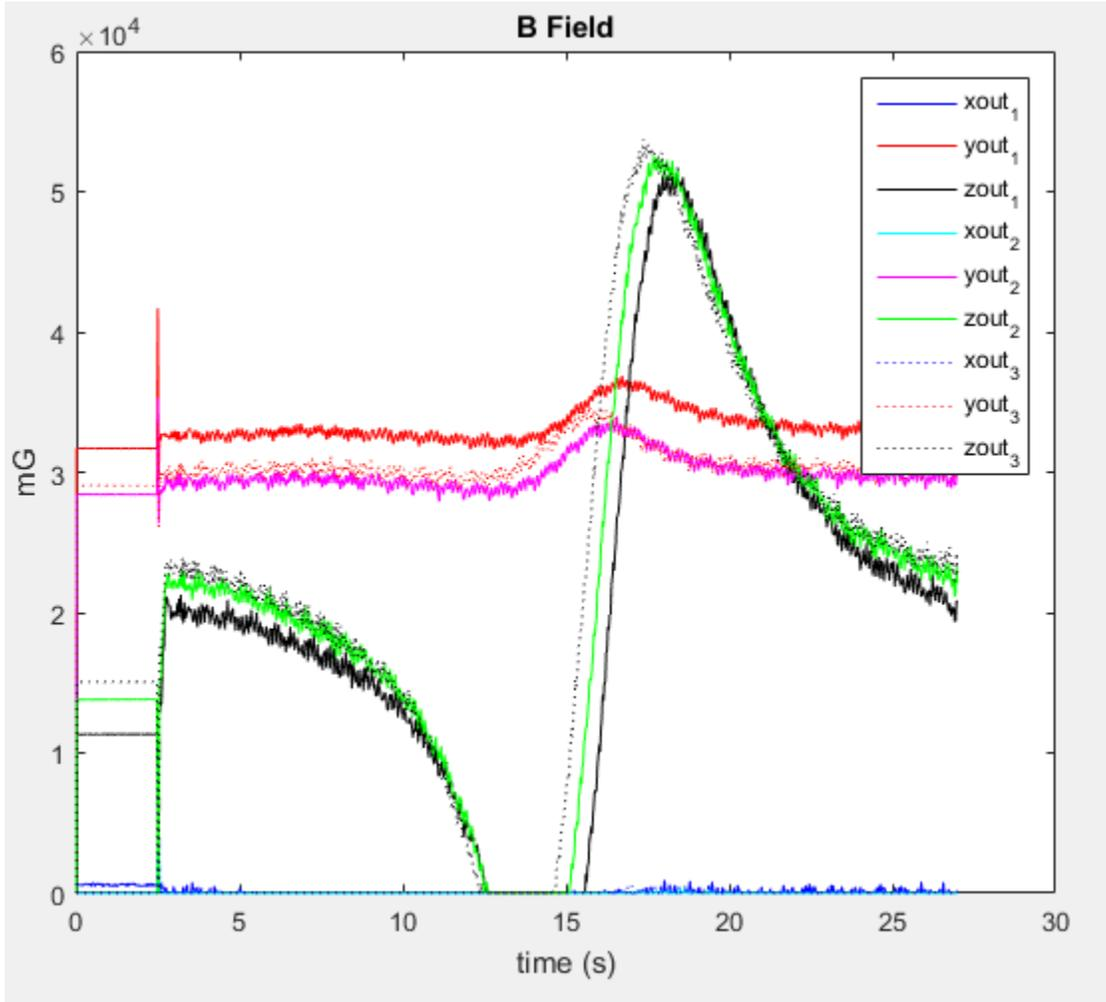
*Figure 3.* Magnetic field data of dipole magnet attached to extending piston of electro-hydraulic actuator. Magnet passes underneath 3, 3-axis Honeywell Anti-Magneto Resistive (AMR) sensors each separated by one millimeter on PCB board, resulting in 9 distinct magnetic field signals. The large disturbance at the beginning and end of the 20 second duration test indicates the 12V DC motor initializing/terminating 10A current draw.
