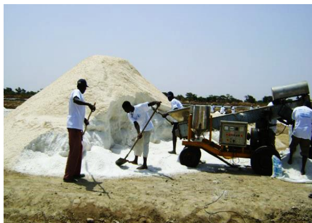
Figure 2. Manual method of salt iodization in a salt production plant in Ndiemou.
