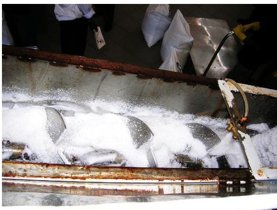
Figure 1. Spraying method of salt iodization in a production plant in Sri Lanka
